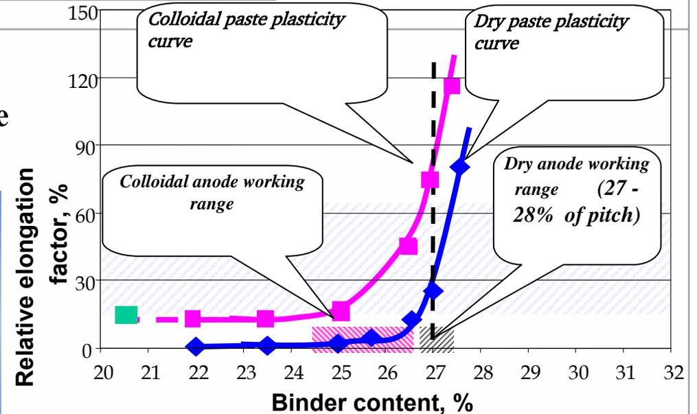
Colloidal anode provides for stability of physical properties when pitch content is close to that of a pre-baked anode - PAH emissions are reduced by over 50%
